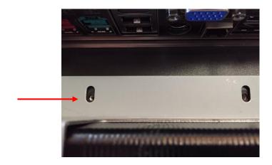
b. Screw Bracket To Kiosk Using 2 Small Black Screws Provided.
