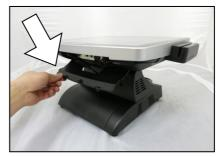
4. Push down IO cover to access IO ports.
