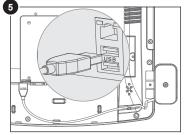
Connect USB A cable to IO port to complete installation.
