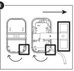
Move bracket, cable and rubber to the other side then close the cover
