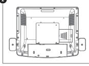
Secure reader to machine with included screw, either on left or right side.
