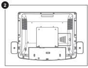
Secure reader to machine with included screw, either on left or right side.
